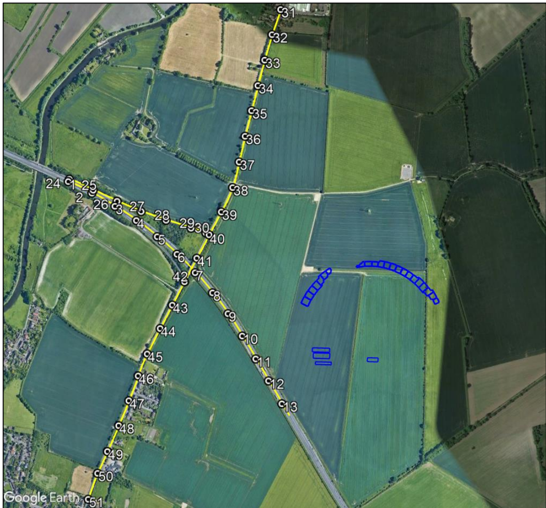
Figure 23 Section of road where solar reflections are geometrically possible
