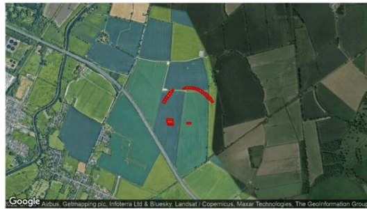
Observer Location Sun azimuth range is 262.5° - 273° (yellow)
